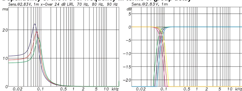
The lower the x-over frequency is the higher the group delay increase is. This leads to a less tight bass impulse.
