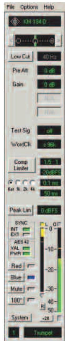
The RCS software control screen for configuring the KM-D digital microphone
