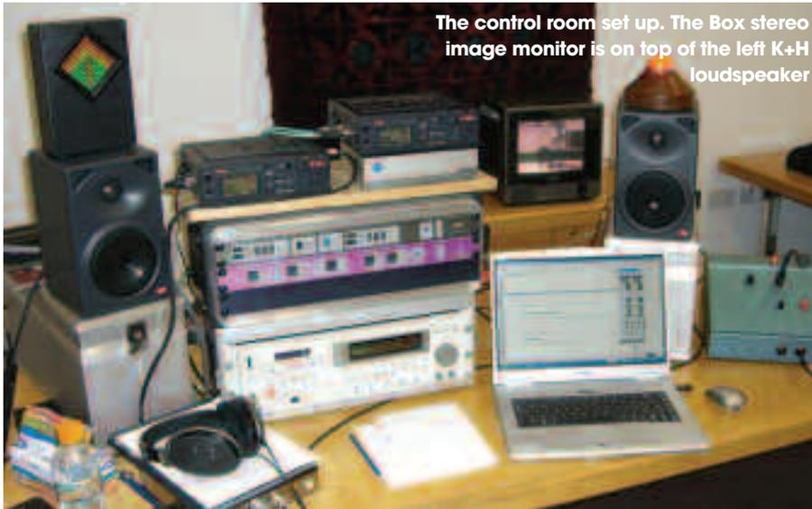
The control room set up. The Box stereo image monitor is on top of the left K+H loudspeaker
